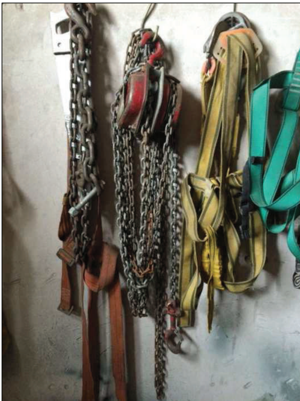
ITEM 1,033 - VISTA DA TALHA MANUAL CAP: 1,0 TON. COM 3,0 METROS
