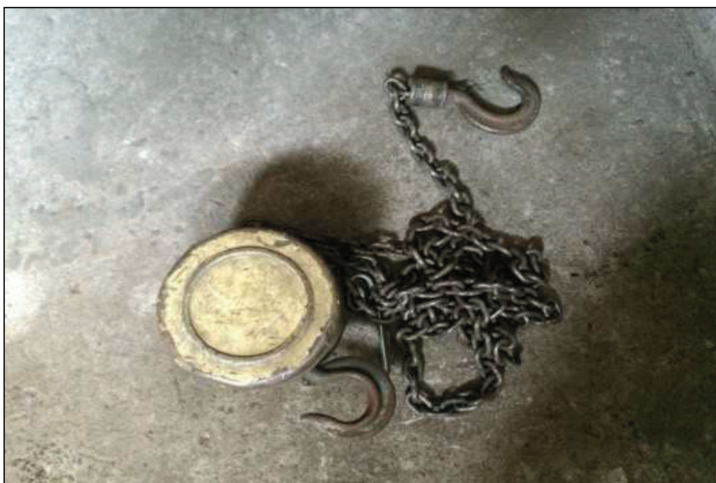
ITEM 1,033 - VISTA DA TALHA MANUAL CAP: 1,0 TON. COM 3,0 METROS
