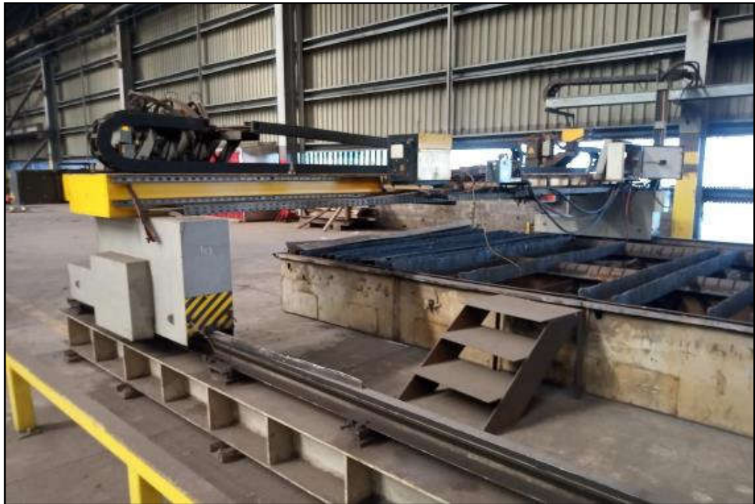
ITEM 1,008 - VISTA DO CORTE A PLASMA ESAB CUTTING SYSTEMS SXE P3 6500
