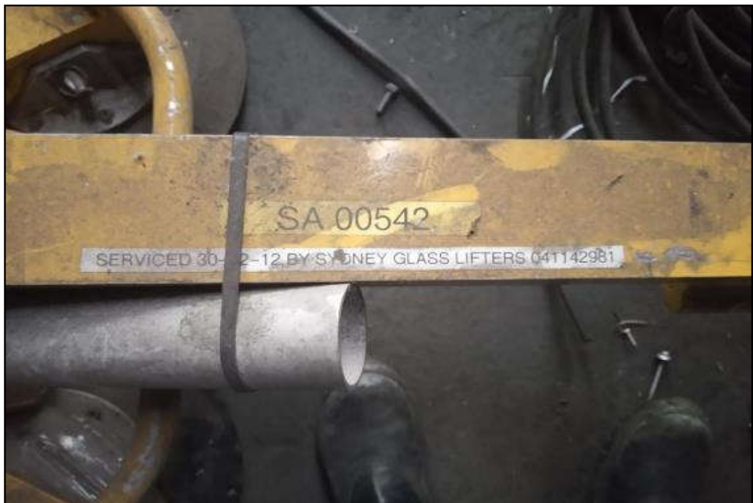
ITEM 1,081 - VISTA DO BALANCIN COM VENTOSA SYDNEY GLASS LIFTERS WLL 320KG
