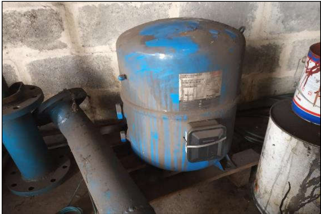
ITEM 1,074 - VISTA DO COMPRESSOR DANFOSS MT125HU4DVE
