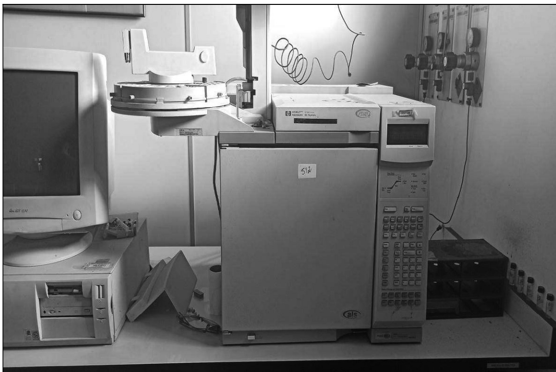
ITEM 1,160 – VISTA DO CROMATOGRÁFO HPLC, FAB. HP, MOD. 6890, SERIES US00023849
