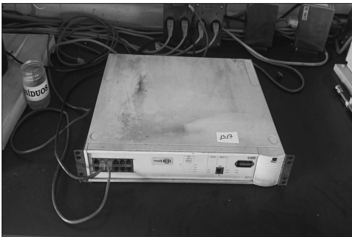
ITEM 1,194 – VISTA DO SWITCH, FAB. 3COM, MOD. SUPERSTACK II 1000, 12 PORTAS
