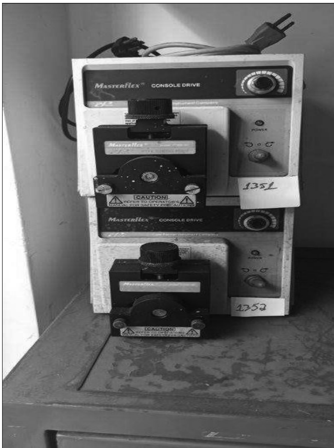
ITEM 1,200 – VISTA DO PTFE TUBING PUMP, FAB. COLE PARMER, 77390-00
