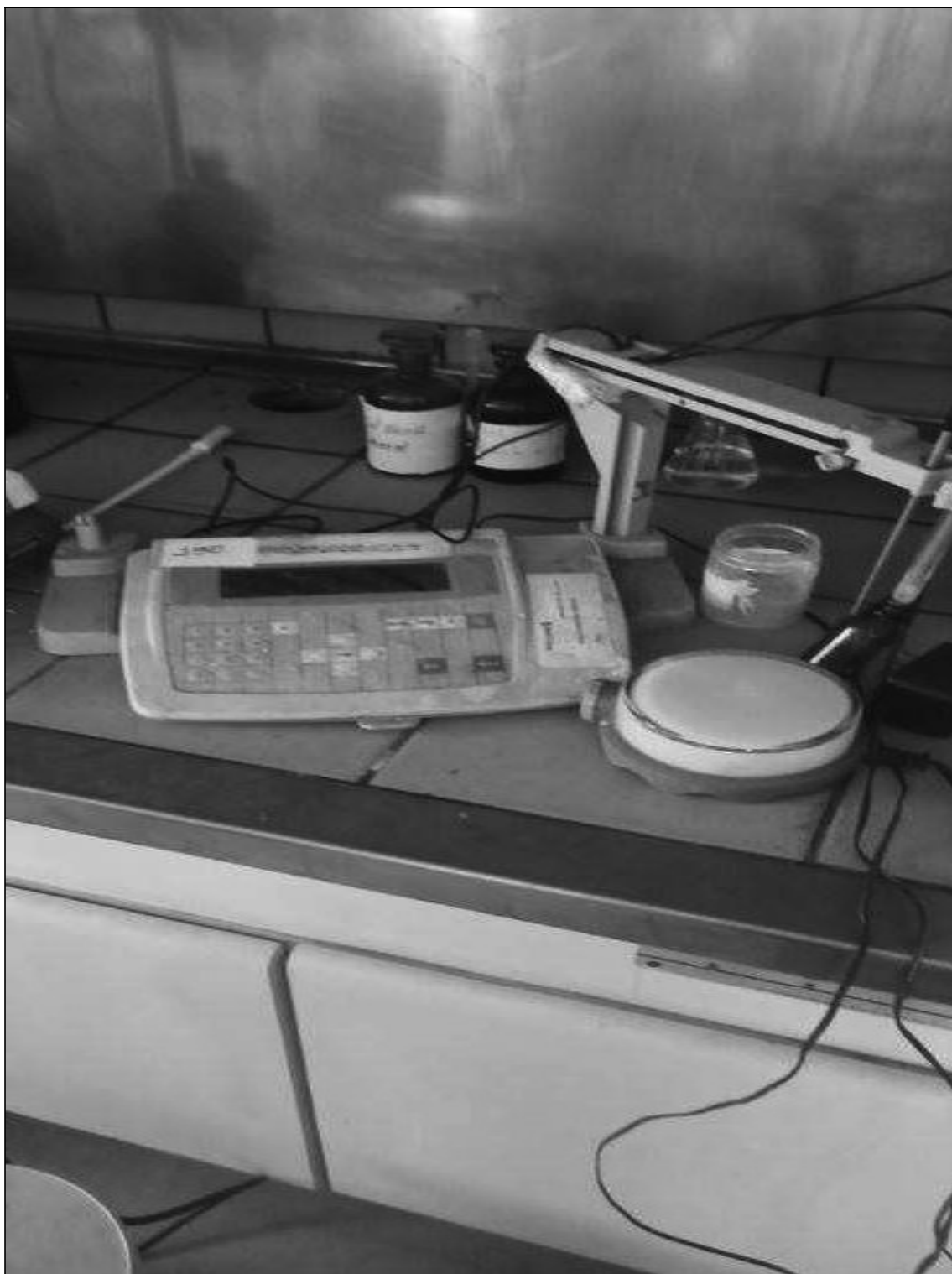
ITEM 1,128 – VISTA DO PH METRO, FAB. METLLER TOLEDO, MOD. MA235
