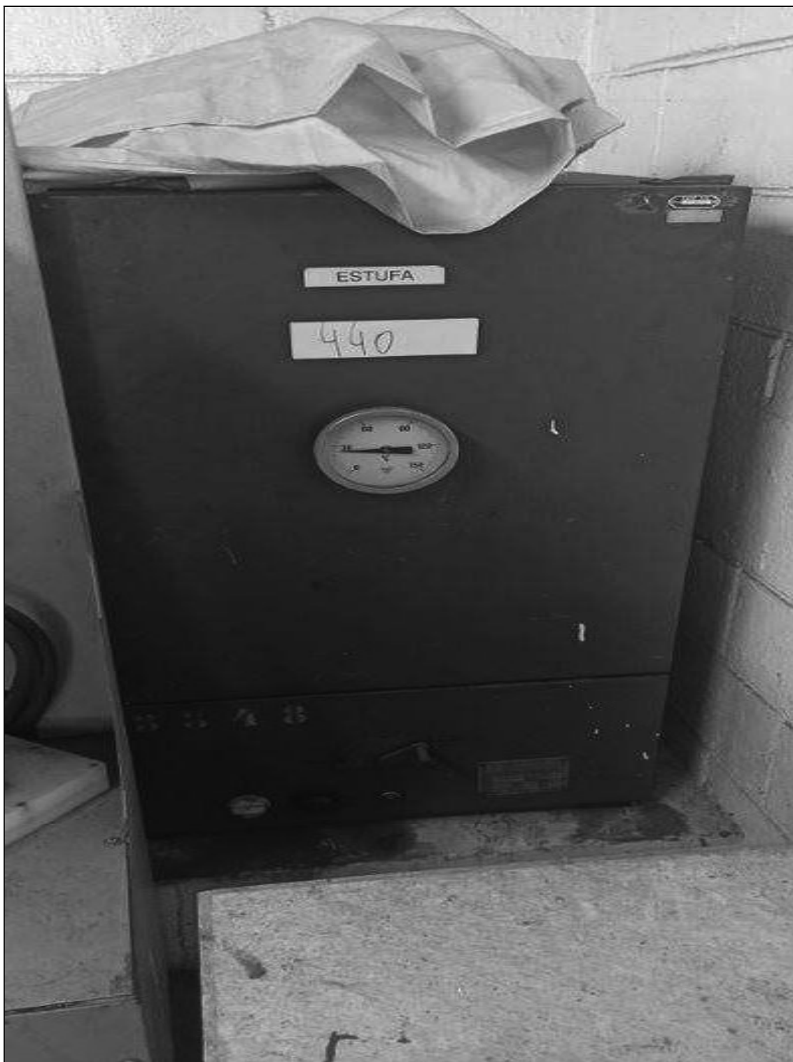
ITEM 1,146 – VISTA DA ESTUFA ELETRICA, FAB. SIGMA, MOD. EERE-100, 15 KW, DIM. 600X600X1200 MM
