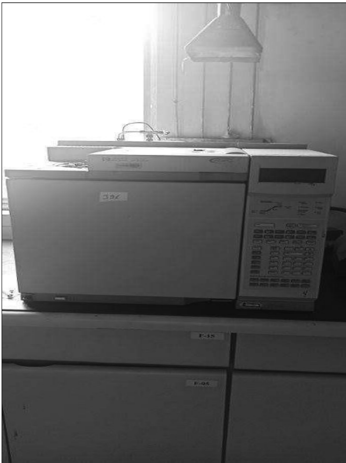
ITEM 1,129 – VISTA DO CROMATOGRFAO EG A GAS, FAB. HP, MOD. 6890, SERIES V500024076
