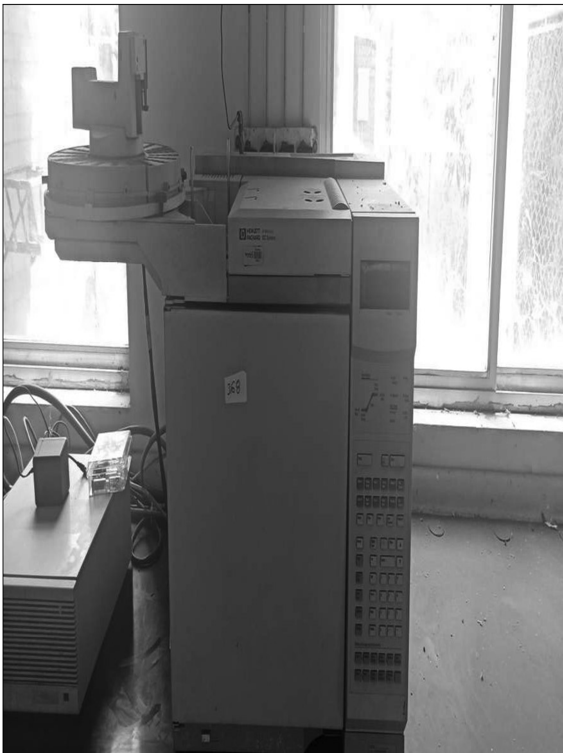
ITEM 1,111 – VISTA DO CROMATOGRÁFO EG A GAS, FAB. HP, MOD. 6890, SERIES US00002836
