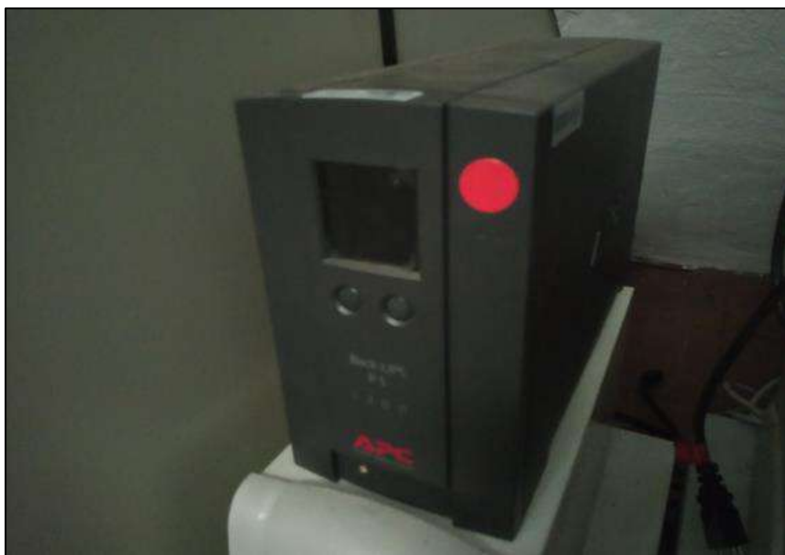
ITEM 3,012 - VISTA DO NOBREAK APC BACK UPS RS 1300
