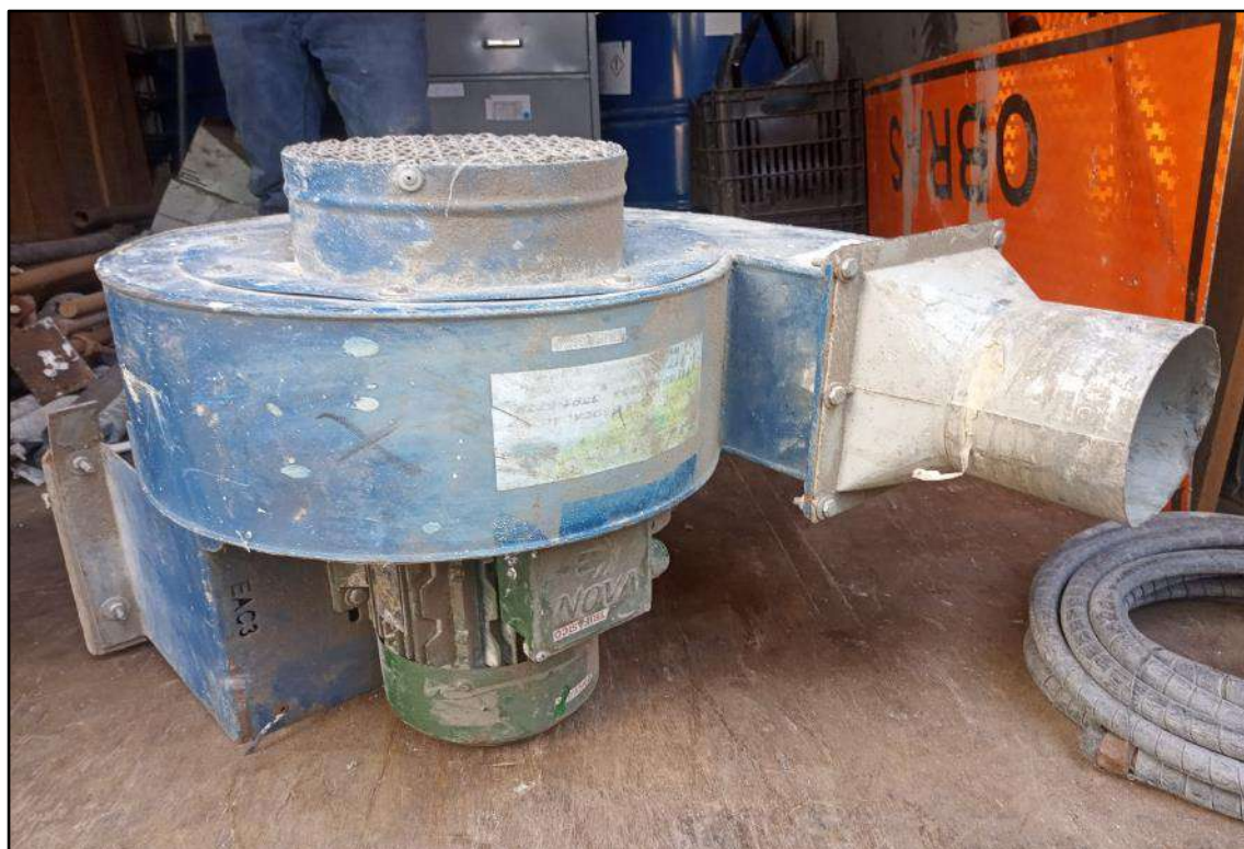
ITEM 1,026 - VISTA DO EXAUSTOR INDUSTRIAL
