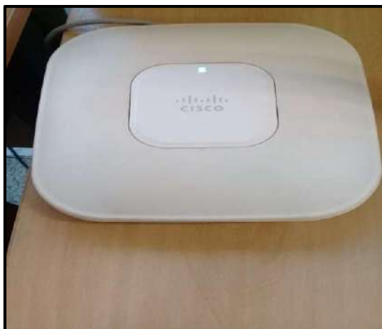
Access point Cisco
