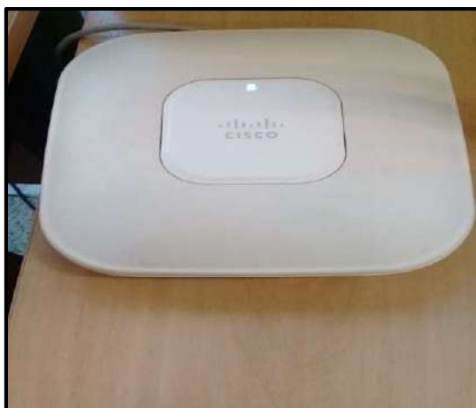
Access point Cisco
